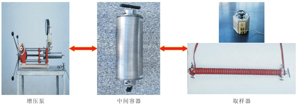
图 3 样品密封性检查照片 Fig.3 Test of Sealing for the samples
