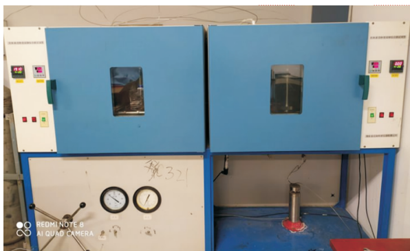
图 5 准噶尔盆地吉木萨尔页岩油岩心 CO 2 吞吐实验装置 Fig.5 Experimental device of CO 2 huff-and-puff in Jimsar shale oil cores of Junggar Basin
