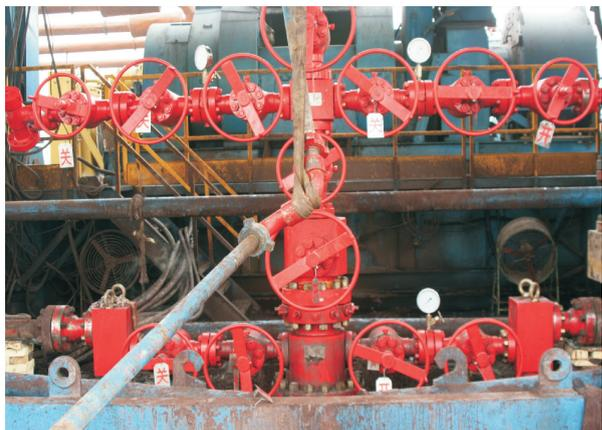
图7 库东3井油管头与压井和节流管汇连接
